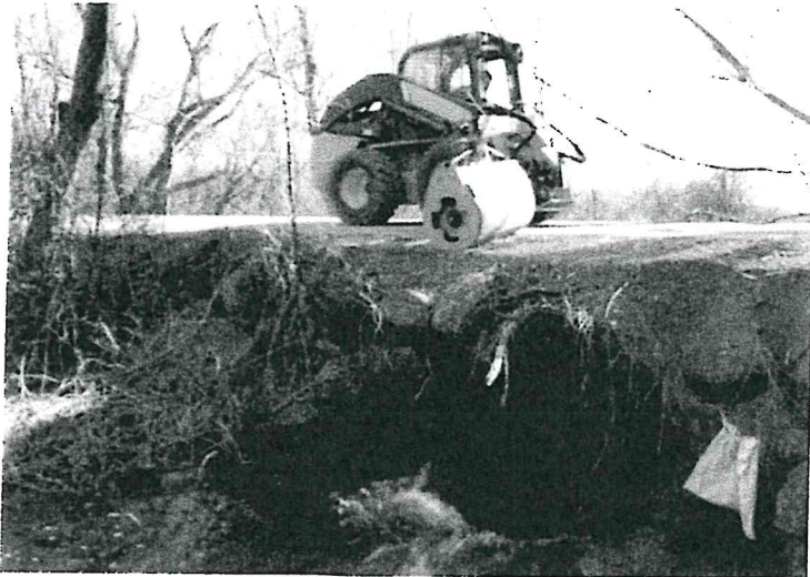
Offset feature allows operator to stay on the road while rolling and compacting shoulders and ditches.
