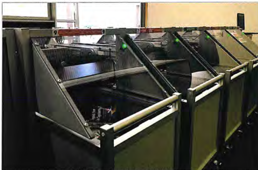
9-bin sorting system installation.
