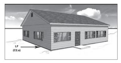
**Building Description** 1 floor on slab (see EC, Diagram 1A)
