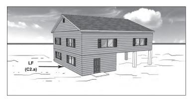
Building Description 1 floor with finished or unfinished enclosed area (see EC, Diagram 6)
