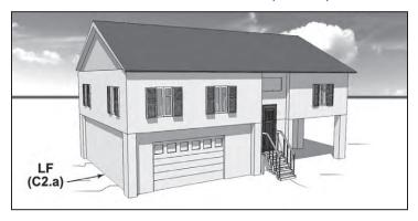
**Building Description** 1 floor Mid-Level Entry with unfinished enclosure (see EC, Diagram 6)
