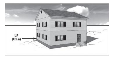
**Building Description** 2 floors on raised-slab-on-grade or slab-on-stem-wall-with-fill (see EC, Diagram 1B)
